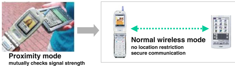
Fig. 2. Establishing a wireless connection by measuring the signal strength
